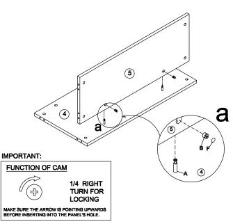
NOTE: CAP 'E' INSTALL ONTO 25MM PANELS. CAP 'F' INSTALL ONTO 18MM PANELS.
